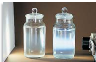
FIGURE 4 A beam of light distinguishes a colloid from a solution. The particles in a colloid will scatter light, making the beam visible. The mixture of gelatin and water in the jar on the right is a colloid. The mixture of water and sodium chloride in the jar on the left is a true solution.
