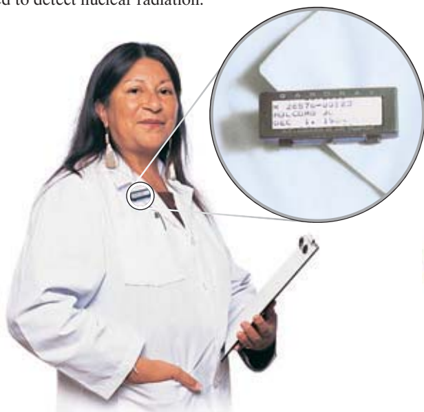
FIGURE 12 Film badges (a) and Geiger-Müller counters (b) are both used to detect nuclear radiation.
